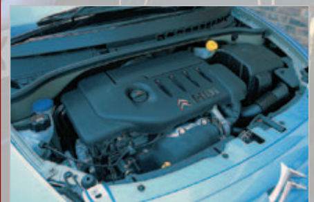
Citroën's 1.4-litre HDi Common Rail engine.
